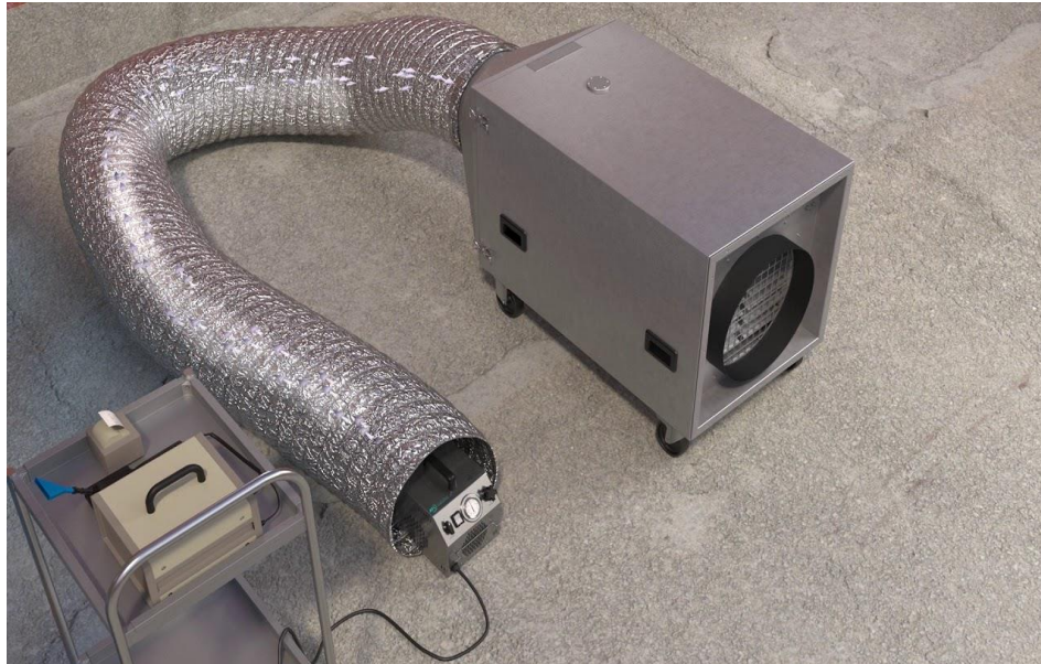
2 Negative air unit set-up to be performance leak tested with mixing chamber.
